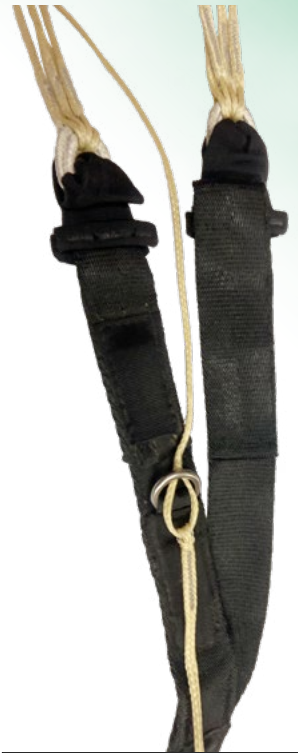
Finding the sweet spot: Here, the locking loop on the steering lines are even with the steering-line ring on the riser.
