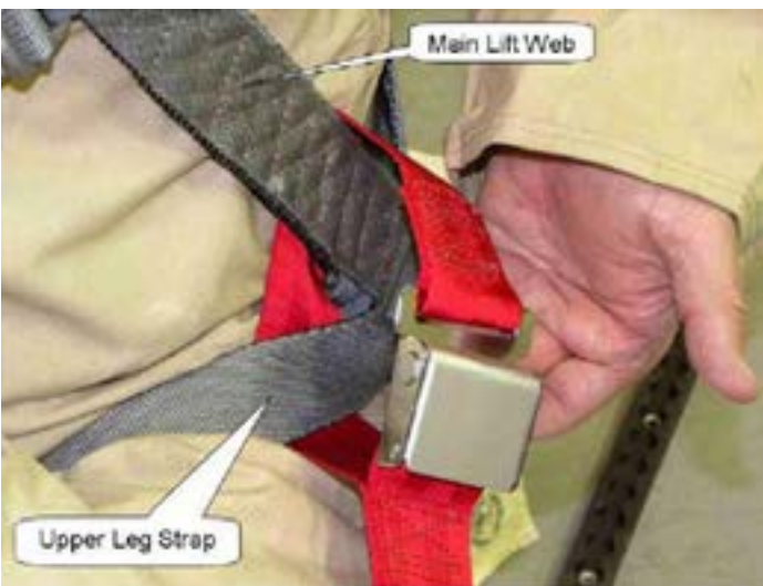
Figure 6. Latch Tether Loop Around Parachute Harness
