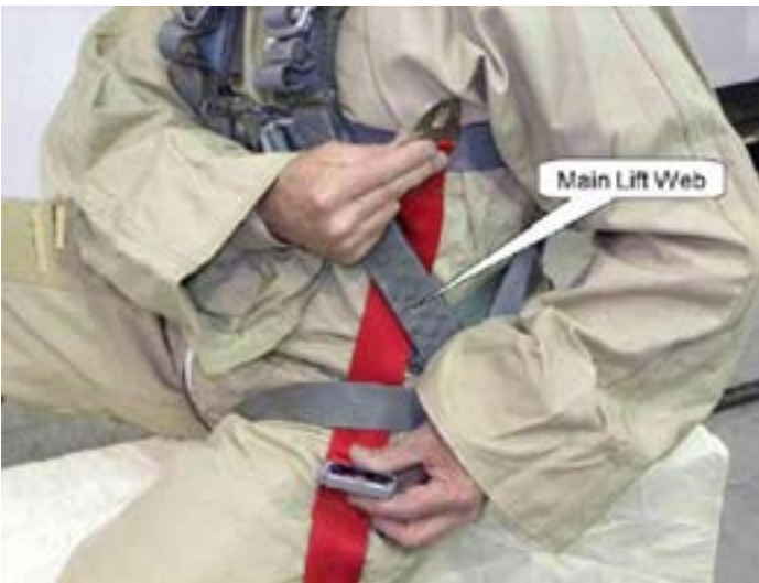
Figure 5. Pass Tether Loop Under Main Lift Web
