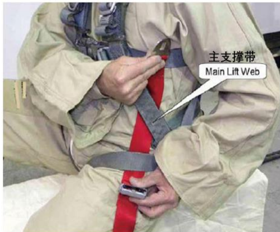
图5 系绳穿过主支撑带 Figure 5. Pass Tether Loop Under Main Lift Web
