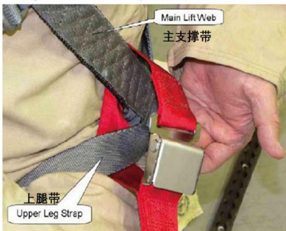
图6 将系绳式安全带扣在降落伞背带上 Figure 6. Latch Tether Loop Around Parachute Harness
