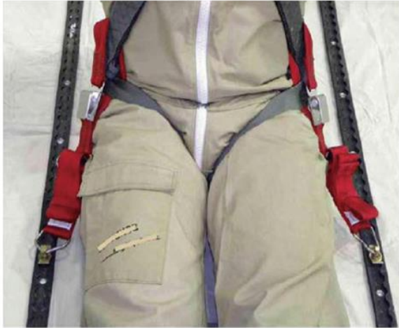
Figure 8. Dual Point, Dual Tether Restraint Configuration For Rear-Facing Floor Seats
