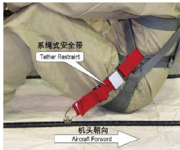
图7 系绳与机舱地板的连接 (对于面朝机尾的机舱地板座椅) Figure 7. Tether Restraint Attachment To Floor For Rear-Facing Floor Seats
