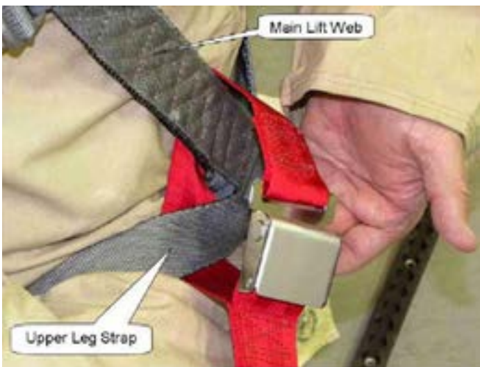
Figure 6. Latch Tether Loop Around Parachute Harness
